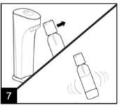
Pull Fizz Infuser and Bottle Assembly forward 45 degrees and slide it off of the machine. Gently shake the bottle and Fizz Infuser assembly to increase carbonation level.
