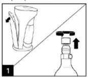
Remove back cover and pin protector as indicated on the instruction attached to the pin protector inside the back panel. Remove seal and twist off cap from CO2 carbonator.
