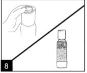
Open the slow release valve on the fizz infuser and pay attention to foam levels as pressure releases. If the foam reaches the top of the bottle close the slow release valve and wait for foam to settle before opening again. If the foam reaches the top too quickly next time shorten your carbonation pushes.
