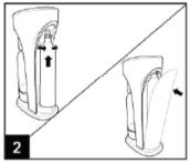
To install CO2 carbonator, insert threaded part of carbonator into unit receptacle and hand-tighten. Replace back cover.
